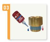
Apply threadlocker along the direction of the vertical thread rotation
