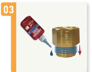
Apply threadlocker along the direction of the vertical thread rotation
